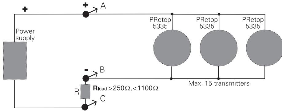
The outputs of max. 15 transmitters can be connected in parallel for a digital HART® communication on 2-wires.
