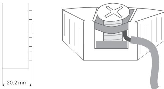
Wires must be mounted between the metal plates.
